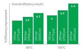
This demonstration shows the impact that fluid formulation and physical characteristics can have on overall hydraulic efficiency. But hydraulic efficiency is not an end goal in and of itself. This additional pumping efficiency can translate into energy savings, as measured by fuel or electricity consumption, or in time to complete a work cycle in hydraulically powered equipment.
