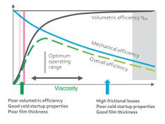
Mechanical losses are highest when fluid viscosity is high and volumetric losses are highest when fluid viscosity is low. Viewing these two curves on the graph illustrates a viscosity range for optimal efficiency. Because hydraulic fluid viscosity is high at low temperatures and decreases as the fluid temperature rises, staying within this optimal operating range is not simple. Specially formulated hydraulic fluids can reduce the magnitude of these
