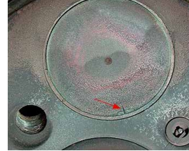
Figure 7 A cracked valve
