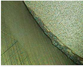
Figure 5 Piston detonation build-up
