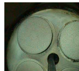
Figure 3 Valve deck ash layer
