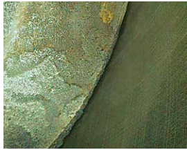
Figure 4 Piston crown carbon build-up
