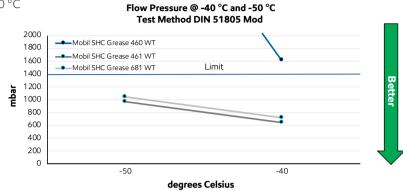
Customer Benefit: Increase wind turbine reliability even in extreme temperatures down to -50 °C. Only half the pressure needed to pump the grease @ -40 °C (DIN 51805)
