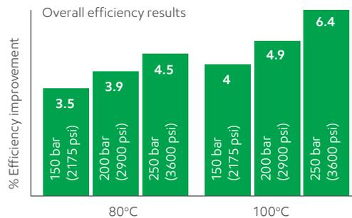
This demonstration shows the impact that fluid formulation and physical characteristics can have on overall hydraulic efficiency. But hydraulic efficiency is not an end goal in and of itself. This additional pumping efficiency can translate into energy savings, as measured by fuel or electricity consumption, or in time to complete a work cycle in hydraulically powered equipment.
